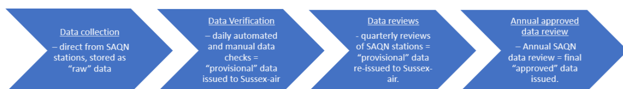
Figure C.1 – Sussex Air Quality Network data validation process
