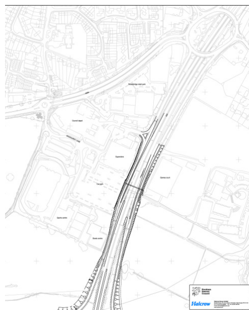
Initial design of overlapping sliproads to be finalised at the planning application stage
