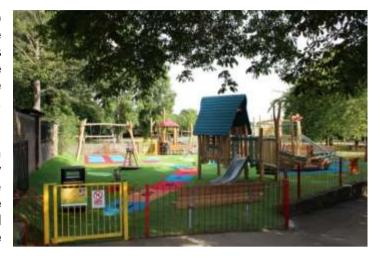
A clearly recognisable boundary to the activity area, created through planting and ground formations etc. If there is a road allowing 30 MPH or more travel speed within the buffer zone, then the activity area must be enclosed by a sturdy, but attractive fence, 0.9-1.2m high with access through an inward opening, self-closing gate of width, 1.2m.
